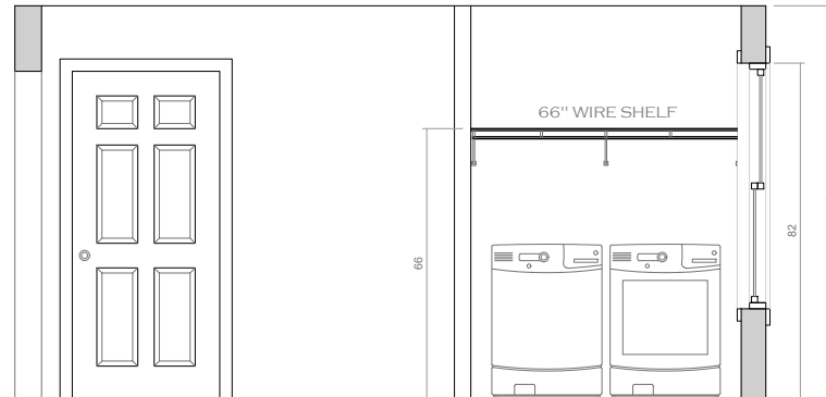
INTERIOR ELEVATION @ WASHER & DRYER
