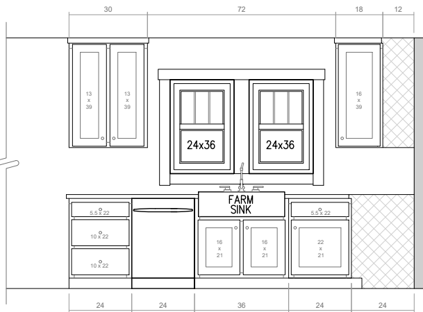
KITCHEN ELEVATION @ SINK / DISHWASHER
