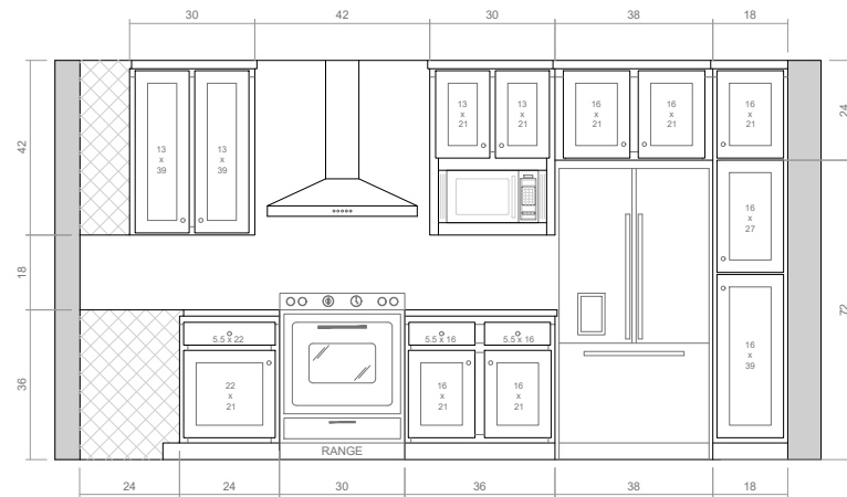
KITCHEN ELEVATION @ OVEN / REFRIDGERATOR
